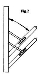
If restrictors 'B' are fitted and it is necessary to open beyond this point, push the restrictor in and slightly down to lock in position. The sashes can now be slid fully open. To restrict the windows again, unclip the restrictor.
